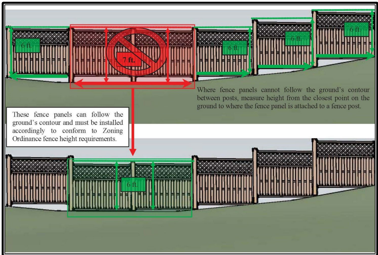
Figure VII-62 Measurement of Pre-constructed Fence Panel Height on Uneven Ground
